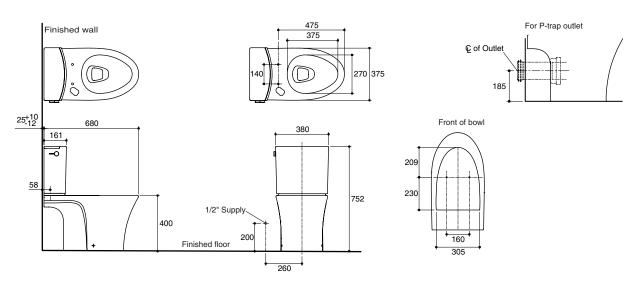
Note: The recommended dimension for installation can be adjusted according to user preferences and layout Kohler Co. reserves the right to make changes in product characteristics, packaging, or availability at anytime without notice
